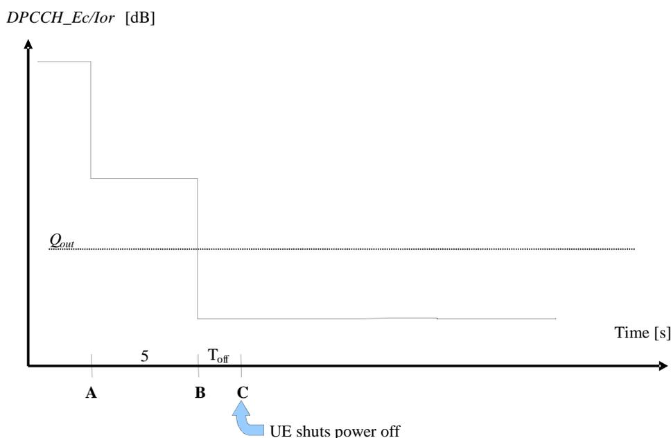
Figure 4.2.11.2-1: Conditions for out-of-synchronization handling in the UE
